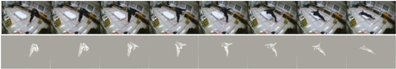
Fig. 2. The person falls on the bed and GMM is applied to separate the moving part of the image in 40 frames with 5 step.
