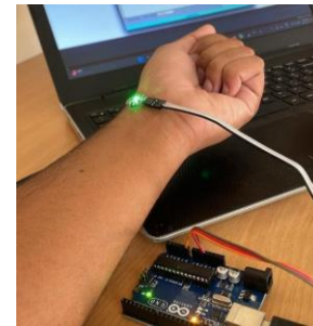
Figure 5. PPG Sensor Placement on Wrist
