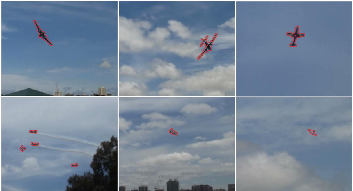
Fig. 4. Airplane Detection. Airplanes' contours and centers are shown by red color
